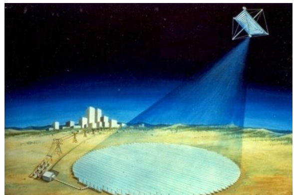
SSP platform transmits energy to ground antenna where it is then provided to electric utilities.
