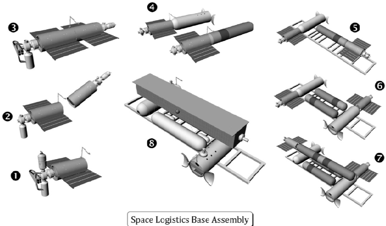
1. First space construction station is deployed to orbit using the Shuttle-derived spacelifter. Assembly crews are transported to the station using the Gen. 1 passenger spaceplane while the Gen. 1 aerospaceplane delivers cargo containers and the first space tug. First space station achieves operational status.
